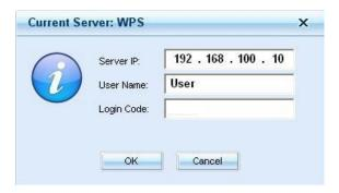
4.8 Enter the **LOGIN CODE** from the projector screen to start sending the display signal
